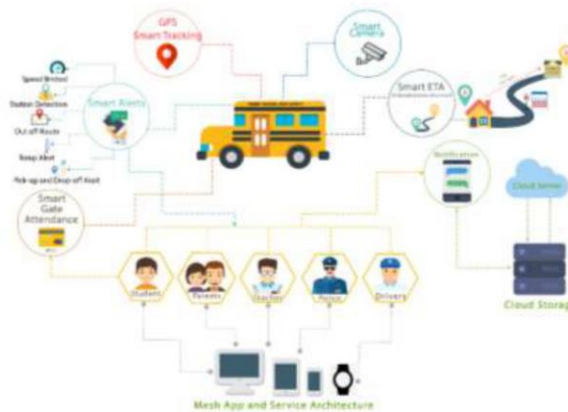
Fig. 1. Process of the smart bus management system using mesh app and service architecture.
